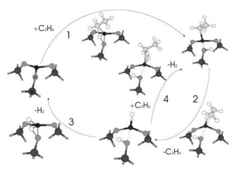
**Figure 10.** Optimized stationary structures for the dehydrogenation reaction of ethane over the (101)-3bridge model catalyst. The reaction steps are (1)  $\sigma$ -bond metathesis C—H activation of ethane, (2)  $\beta$ —H transfer to chromium with subsequent loss of ethene, (3)  $\sigma$ -bond metathesis O—H activation with subsequent loss of H<sub>2</sub>, and (4)  $\sigma$ -bond metathesis C—H activation of ethane with subsequent loss of H<sub>2</sub>
