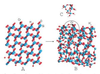
**Plate 1.** Systematic preparation of Cr–silica surface models using simulated annealing. A: The unrelaxed surface with Cr, H and O added B: The fully relaxed slab model following simulated annealing and optimization C: Cluster model with H-terminated dangling bonds
