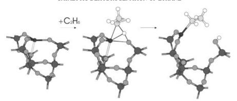
**Figure 12.** C—H activation by  $\sigma$ -bond metathesis, reaction (1), on the (111)-3bridge model catalyst. A silanol group is formed, and optimization at the QM–MM level of theory makes the Cr—silanol distance increase to more than 5 Å as the surface relaxes. The unreacted chromium site is optimized at the QM-MM level, and the transition state of C—H activation is optimized at the cluster QM level. For details concerning optimization of the ethyl complex, see the text
