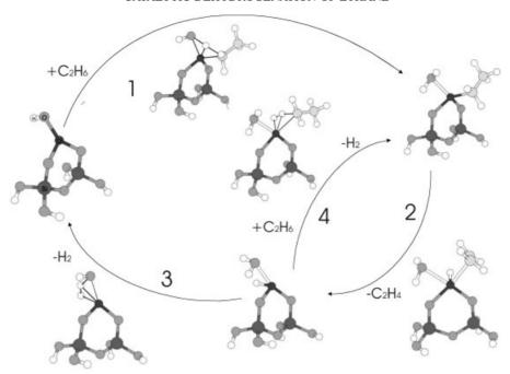
**Figure 4.** Optimized stationary structures for the dehydrogenation reaction of ethane over the DeRossi-1 model catalyst. The reaction steps are (1) C—H activation of ethane, (2)  $\beta$ -H transfer to chromium with subsequent loss of ethene, (3) Cr—O formation with subsequent loss of H<sub>2</sub> and (4) C—H activation of ethane with subsequent loss of H<sub>2</sub>
